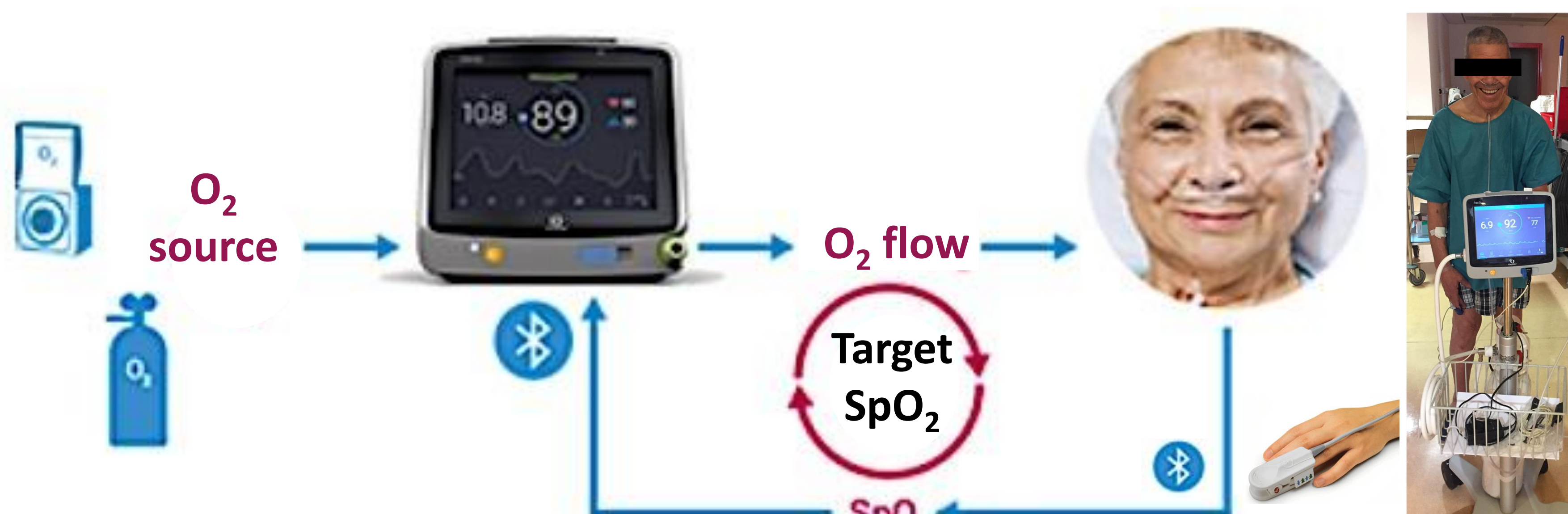
Fig. 1: FreeO2 ® , an automatic oxygen titration device that adjusts oxygen flow rate to a predefined targeted SpO 2
